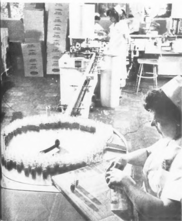
After purification and refining, aureomycin is then packaged in its 16 forms. Here vials containing aureomycin capsules start on their journey to the capping machine. The worker in the foreground checks each vial to see that each contains the proper number of capsules.
