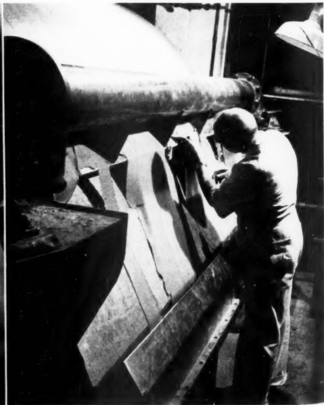
After the Streptomyces aureofaciens mold which produce aureomycin, has been grown in huge tanks under ideal growing conditions, the resulting material is put through a giant filter in one of the early stages of extracting the antibiotic drug.
